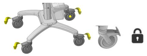
2. To unlock the trolley wheel, push the wheel brake up.
