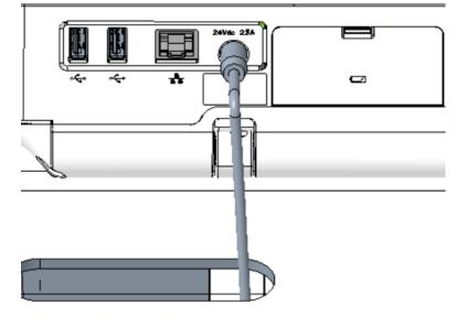
3. Plug the male end of the power cord (2) into an AC outlet.
