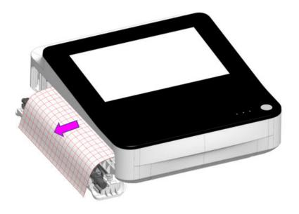
4. Push both ends of the printer door to close it and verify that the unit closes.
